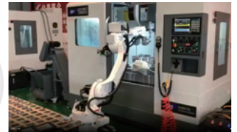
CNC Milling Machine Tending from Front or Side
